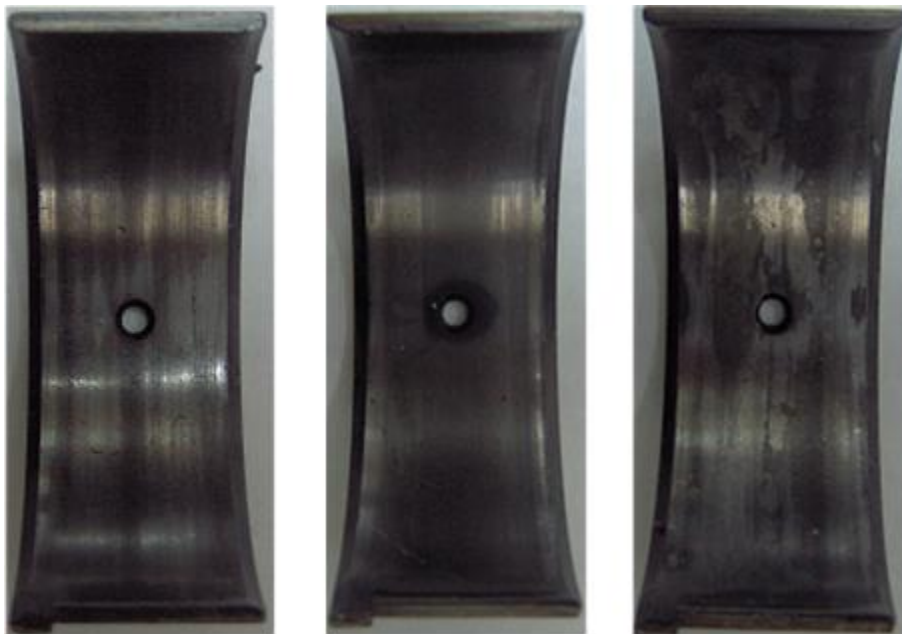
Fig.9 Bearings with various eccentricity values after rig tests
